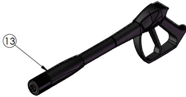
GUN & WAND 5075PSI, 3/8 QC(M)IN X M22(F) OUT PART NO. 7103240
